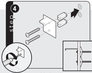
Attach bracket with mounting hardware provided.
